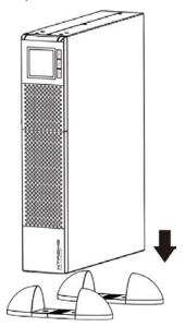
Carefully lower the UPS into the brackets as shown
