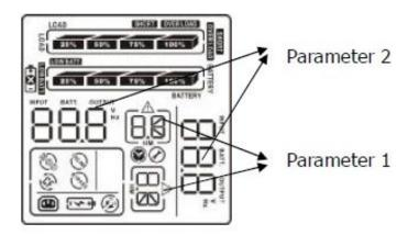
There are two parameters to set up the UPS. **Parameter 1:** for program alternatives –
