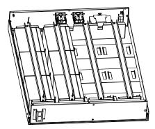
**Note:** To install the second string of batteries, repeat the same procedure on the right side of battery box.
