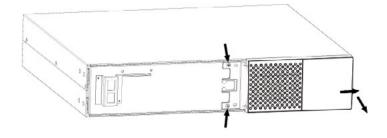
Step 4: Remove the metal top cover of the battery box by unscrewing 8 screws present on the two sides (4 on the right side and 4 on the left side), 3 screws on the top and 4 screws on the back side.
