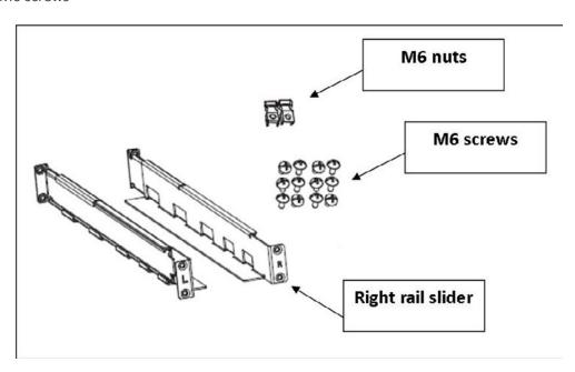
Step 1 Use 4 screws to mount right and left rail sliders in front of rack.
