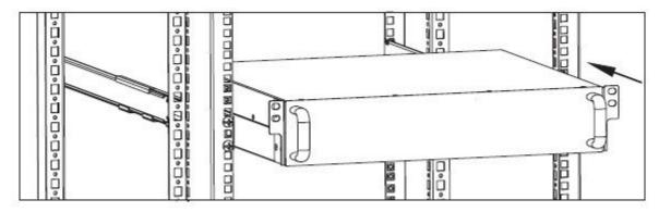
Step 5 Fix the UPS in position with screws.
