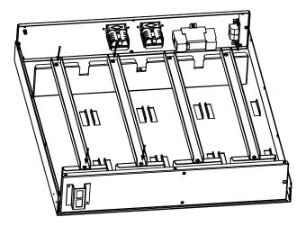
**Note:** To install the second string of batteries, repeat the same procedure on the battery hold down brackets on the right side of the battery box.
