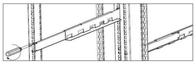
Step 3 Place the nuts in the proper location in the rack based upon height of UPS.
