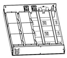
Note: To install the second string of batteries, repeat the same procedure on the right side of battery box.
