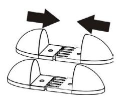
Inter-connect the tower brackets that shipped in the box with the UPS
