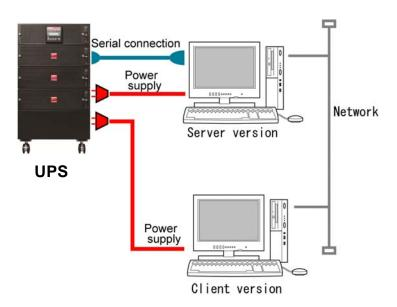
In this case, the computer connected to the UPS using a serial connection (including contact connection) is referred to as a **server version**, and all other computers are referred to as **client version**. (Server and client or client and client must be connected via a network.)
