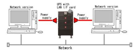
If the UPS has a LAN interface card and is connected to a network, all computers on the network are referred to as **network version**. (There is no distinction between server and clients.)
