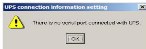
In this situation, confirm that the serial cable is properly connected, UPS power is turned on, and that other applications are not using the same serial port. Retry automatic detection after confirming all of these conditions.
