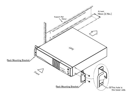
Install the Rack Mounting Brackets to the both sides of the UPS (or the Power Distribution Unit) with the supplied screws, as above.
